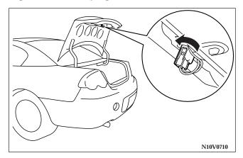
Remove the socket assembly and bulb together by turning it counterclockwise. Remove the bulb from the socket by pulling out.
